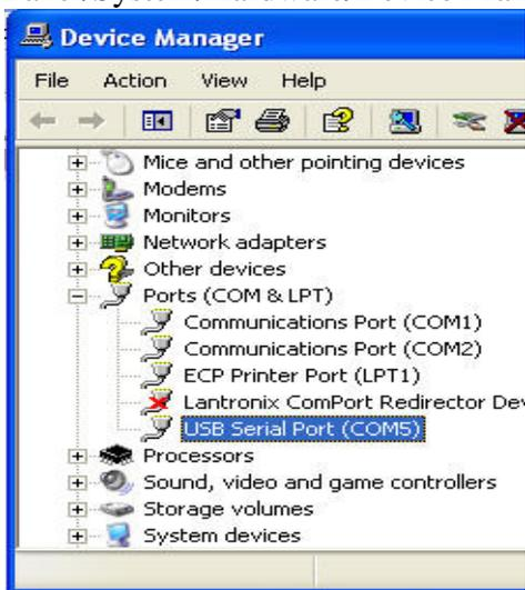
On this computer, the USB-RS232 converter created a virtual serial port COM5. This may be different from PC to PC, so please make sure you check the port-settings on your laptop.
