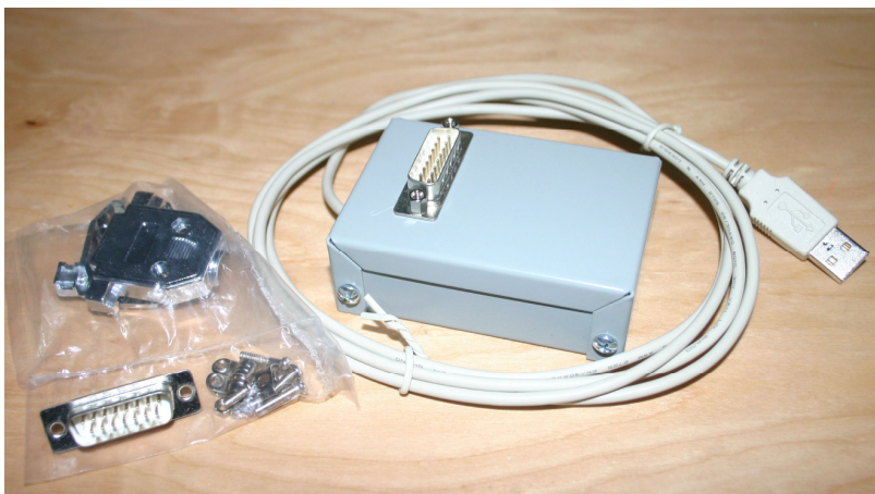
Metal-box version of USB-IO interface
